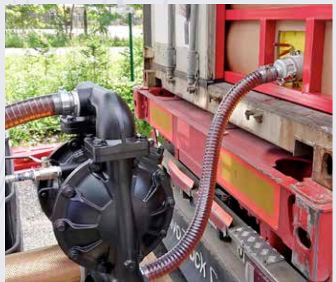
High fluid viscosity reduces pump delivery.
