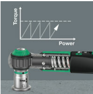
Slide-over mechanism prevents application of excessive torques
