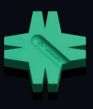
Application: Simply run the tool down the positive side of the Wera magnetiser/demagnetiser and the tool immediately becomes magnetised and is able to hold the screw securely on the blade. To demagnetise the tool, simply run it down one of the four negative sides.
