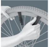
jack, hook into a spoke and pull off the tyre with the second tyre jack. The two tyre jacks can be clicked together and are therefore not lost individually.
