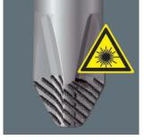
A precisely-focused laser creates a sharp-edged surface structure. This laser treatment results in an edge hardness of up to 1000 HV 0.3. Wera Lasertip "bites" itself into the screw head and prevents any slips out of the recess.
