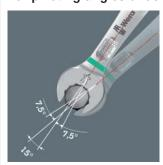
Thanks to the mouth side pivoted by 7.5°, double hexagon geometry and an adjusted application method (placement – screwdriving – turning – turning, etc), even screwdriving challenges allowing a pivoting angle of less than 30° can be solved.
