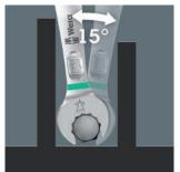
The Joker 6003 combination wrench with its special mouth geometry – an open-end offset by 7.5° and the double hexagon profile – doubles the placement possibilities when repeatedly turning the wrench 180° around the longitudinal axis. Bolts and screw heads can be "accessed" every 15°. The
